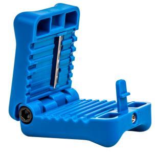
Mid Span Slit Tool is designed to provide easy access to optical fibres in outer jackets and loose buffer tubes. With 6 precision grooves to handle various cable sizes, the sleek ergonomic design allows you to open a fibre jacket or buffer tube without damaging the fibre inside.
